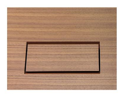
Specially developed single table portals can be optionally integrated into the wood-based table tops. The edges of the segment cut-out and the portal are chamfered in opposite directions so that the gap for the leads looks closed.
