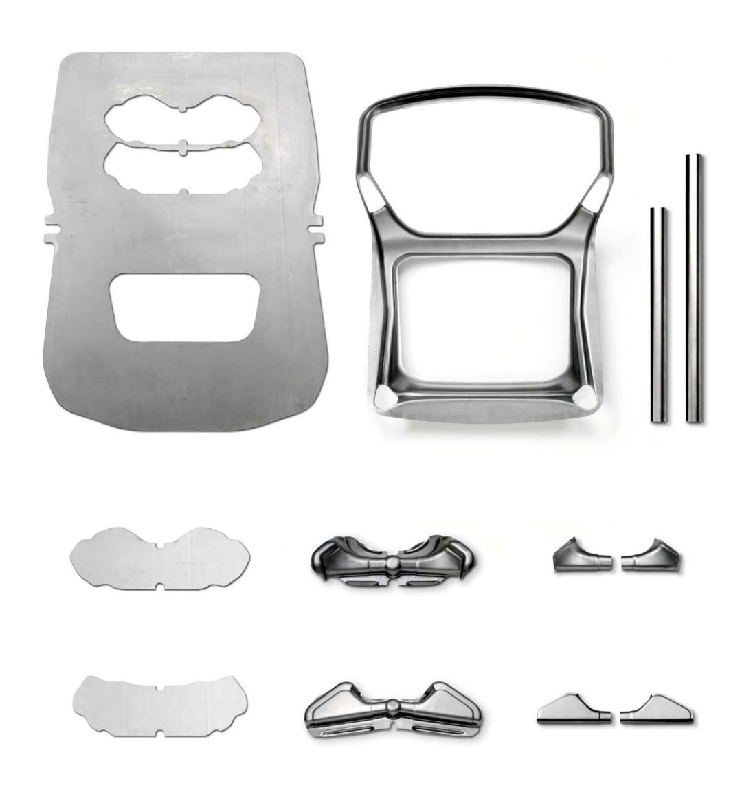
**High tech.** The secret of its elegant appeal lies in the way it's produced. The method is based on car-body manufacture, which has been applied to produce chairs for the first time. Very strong sheet steel is teased into precise forms, welded by robot and powder coated. Then it's combined with the shell to create an attractive piece of furniture.
